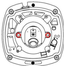
Figure 2-23 Loosen the Lens Set Screws
